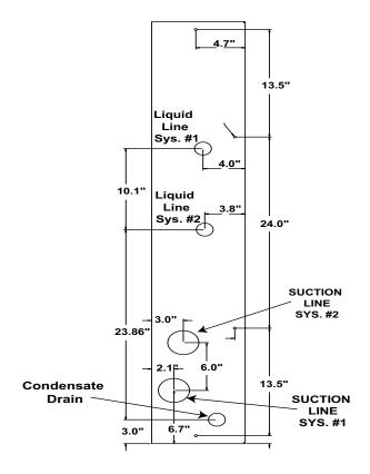
FIGURE 24 - LB600 PIPING CONNECTIONS - END PANEL DETAIL
